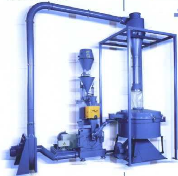
Pulverization plant PU 500 with screen separator
