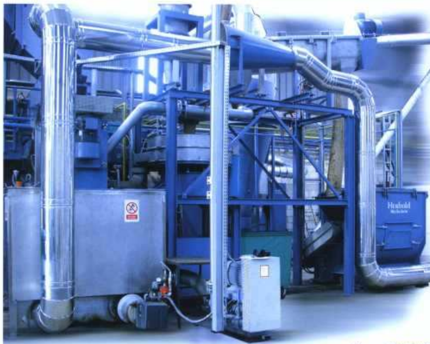
Hot washing plant for PET flakes
