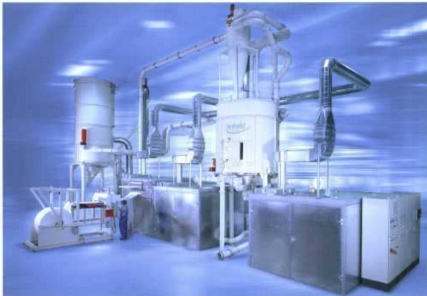
Pulverization plant for cellulose with three SMF 500/1000
